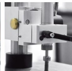
Measuring the hardness of a cylinder with the small cylindrical support ring
